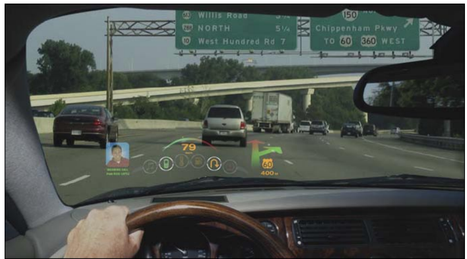
Next generation HUDs further enhance driver safety and convenience with wide field-of-view, full colour images that are artifact free, high contrast and day light readable
